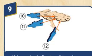
Make sure that the flat edges of these pieces are on the bottom side of the model before attaching them.
