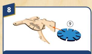
Pay careful attention to the orientation of piece 9. The longest slot on the piece should attach to piece 1.
