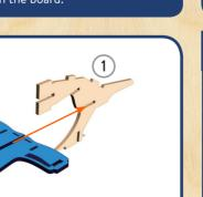
To put the two pieces together, match up the slots on each piece. Slide together.
