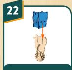
The pegs created by the pieces that connect to the wheel should slide up through the holes on pieces 32 and 33 here.
