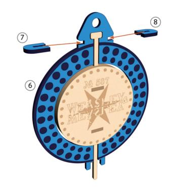
Carefully hold piece 6 in place while attaching pieces 7 and 8.
